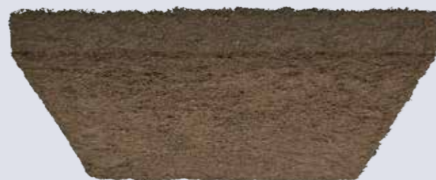
FD Soil Artificial soil with specific gravity reduced to about half of natural soil
